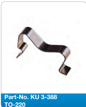
Mat. 0.4 mm, for sheet gauge 1.5-2.0 mm
