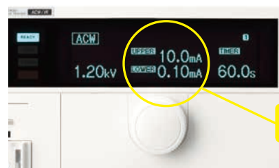
▲ AC Hipot (Withstanding voltage) test settings display (example)
