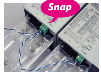
The TP-BUS utilizes a daisy-chain connection. This makes adding power supplies easy and keeps cables neatly together.
